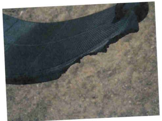
Damaged belt swing seat
