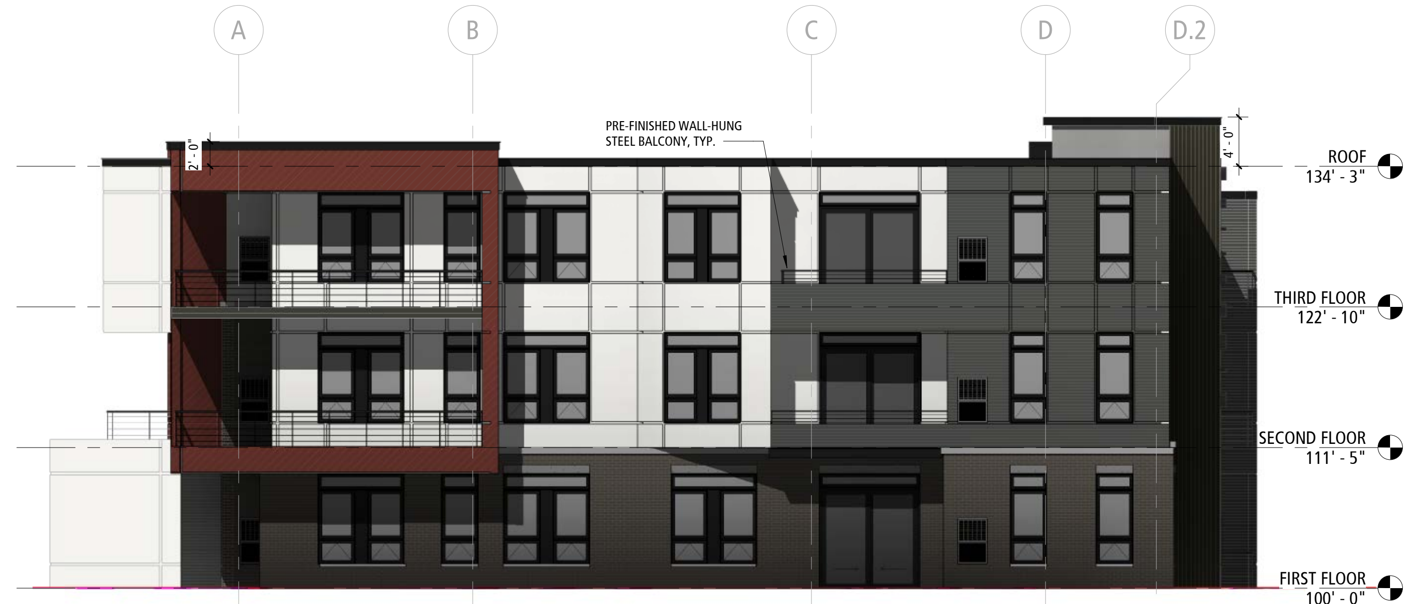
20 OVERALL SOUTH ELEVATION 1/8" = 1'-0" 34 / A101
