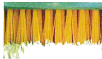
Grooming penetrates the infill by no more than 1/4".
