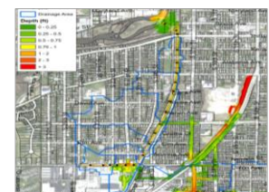
North Priority Area: XP-SWMM 2D analysis showing deficient inlet and conveyance capacity along Union Avenue.
