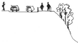
Shared path / two-way bike lane alongside street at the top of the bluff
