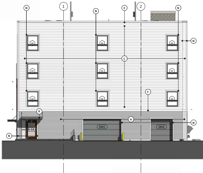
A3 SOUTH BUILDING EXTERIOR ELEVATION SCALE: 1/8" = 1'-0"
