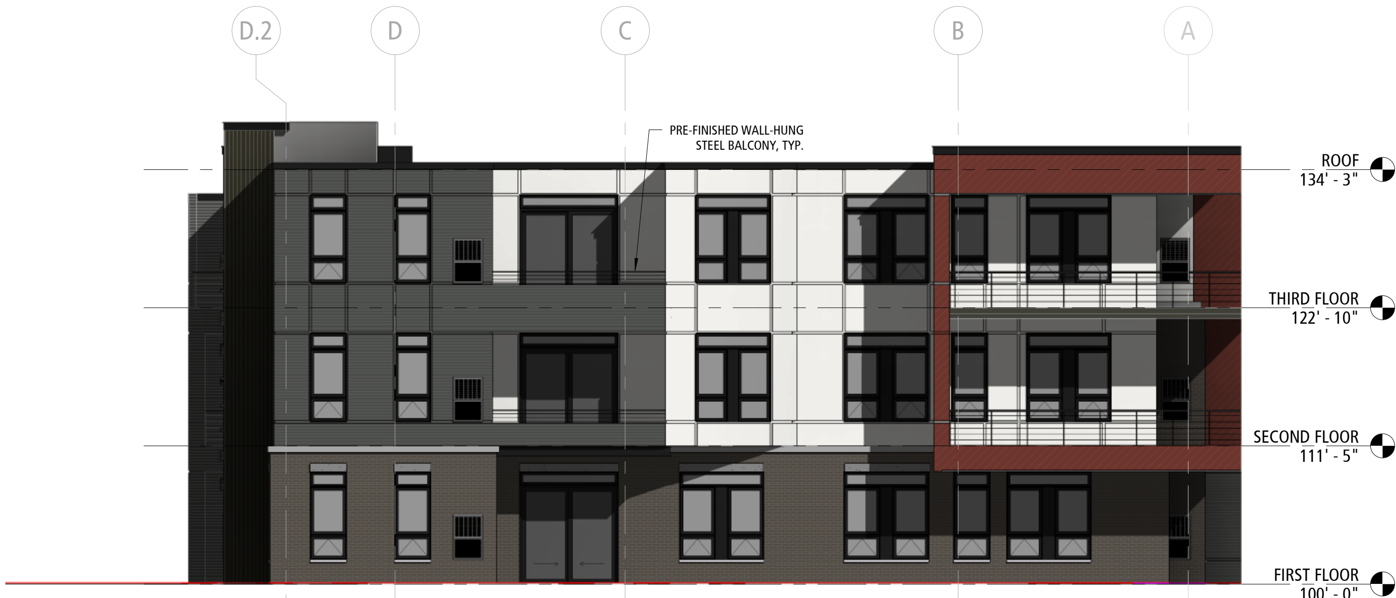
34 OVERALL NORTH ELEVATION 1/8" = 1'-0" 34 / A101
