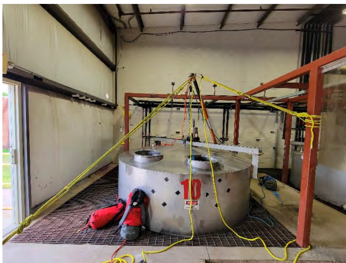
"Gin-pole" created with a leg of our TerrAdaptor tri-pod kit.
