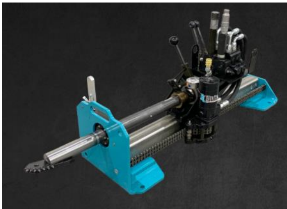
Figure 7-7: Portable HDD – Basement Buddy
