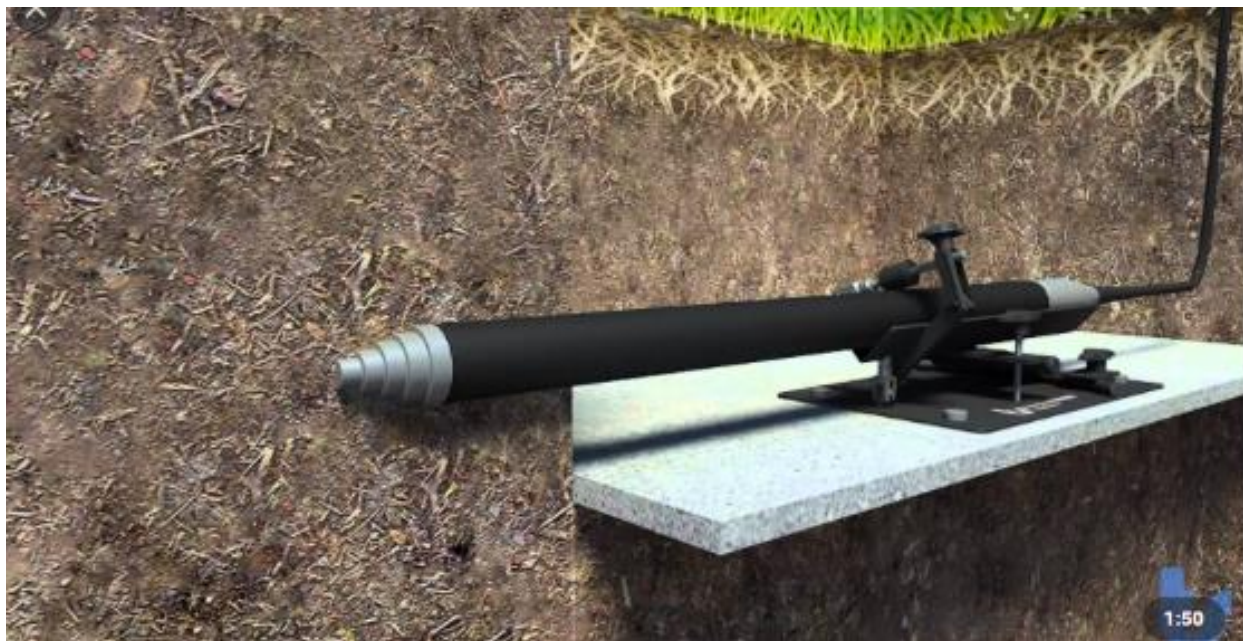
Figure 7-3: Example of a Horizontal Boring Tool
