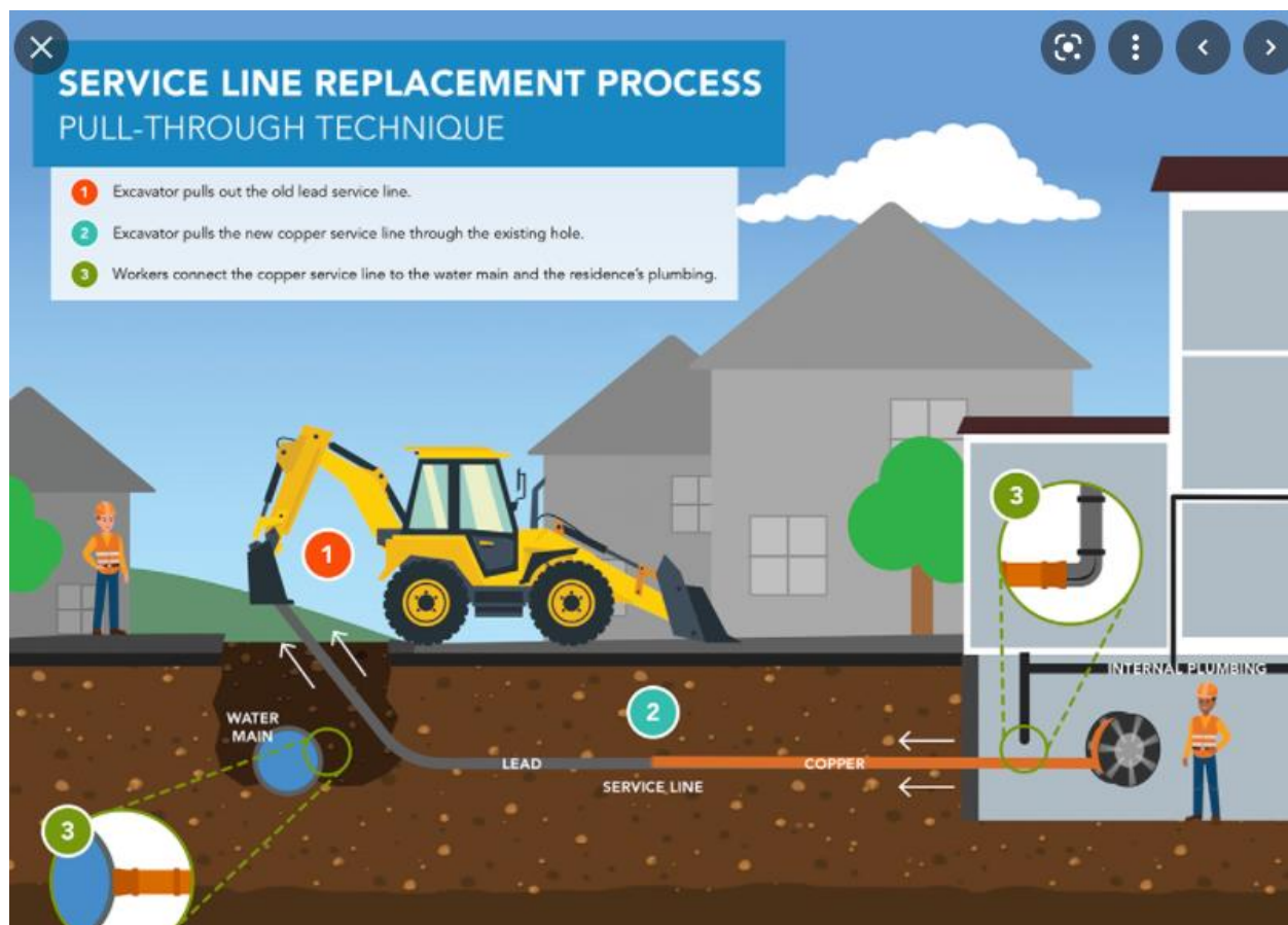
Figure 7-2: Pipe Pulling General Set-Up
