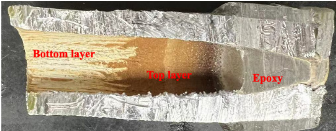
Figure 1. Photograph of the transverse sections of the pipe segment. In this image, a portion of the top layer scale has been removed, which exposes the bottom layer scale.
